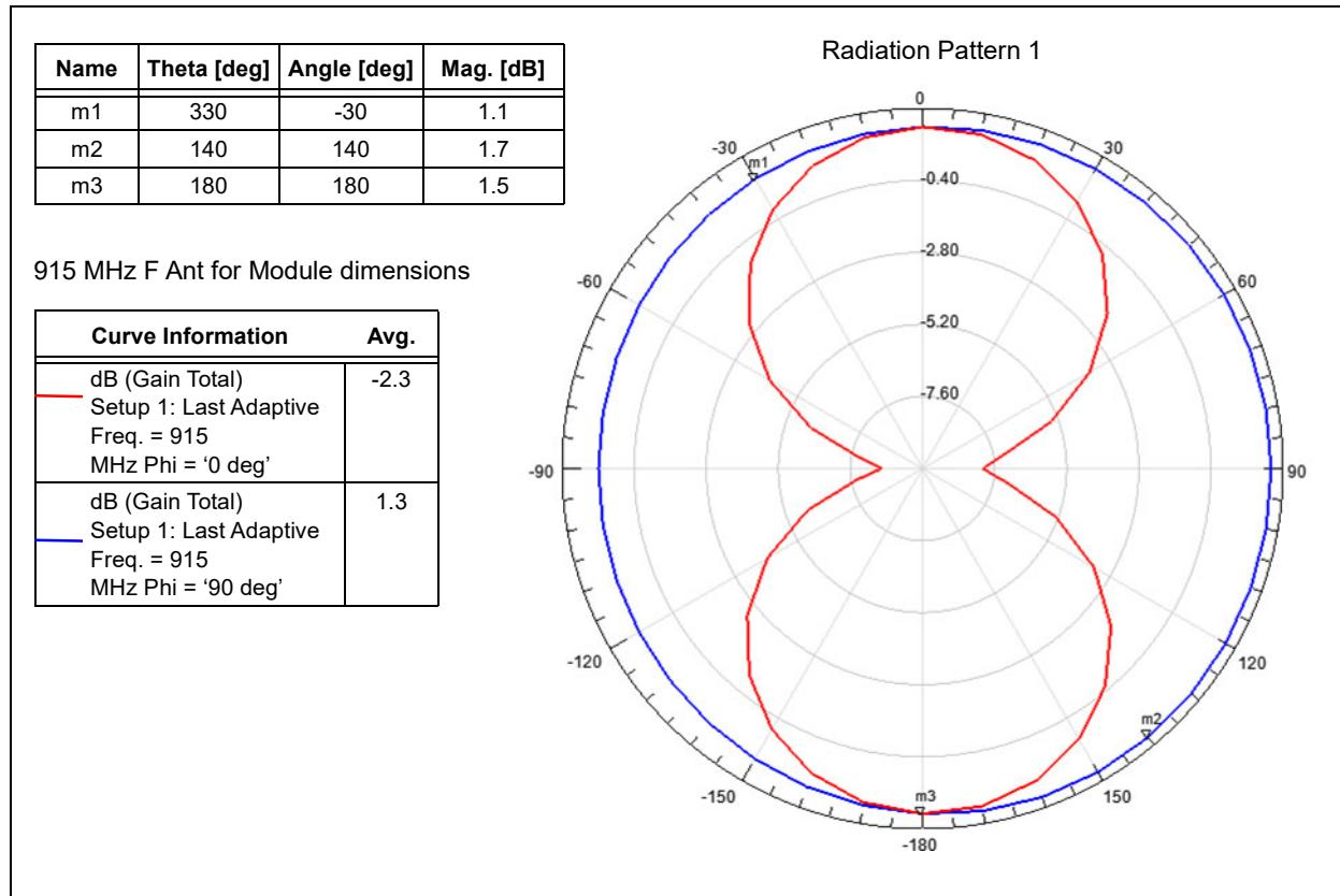
**FIGURE 5-5: SIMULATED THREE-DIMENSIONAL RADIATION PATTERN**
