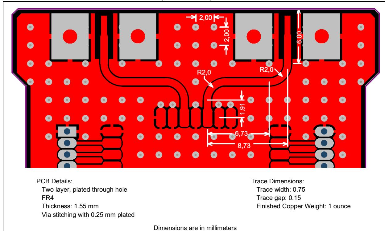
**FIGURE 5-2: RF TRACE ROUTING (BOTTOM LAYER)**
